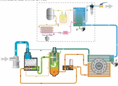
A Intake air B Air/oil mixture **C** Oil D Wet compressed air
